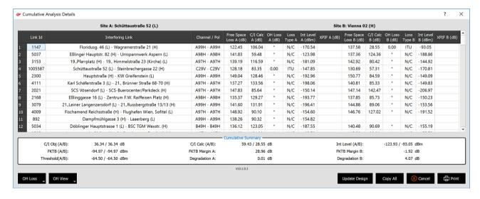
The above window shows each link that contributes to the total interference into the design link.
