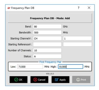
The above example will add the 80GHz band if it doesn't exist, and 10 frequency pairs, separated by the bandwidth of 500 MHz, with channel numbers starting with CH01 through CH20:
