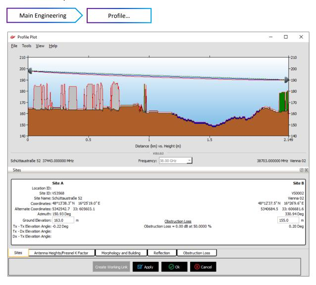
In Profile Menu antenna heights can be optimized, terrain and morphology data revised or modified. Reflection and Anti-Correlation analysis for Space Diversity system design can be performed.
