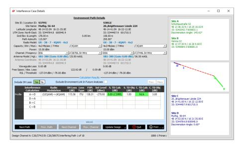
If the **calculated** Single or Cumulative Threshold **Degradation exceeds** the predefined **objective**, the case is reported as an interference case.
