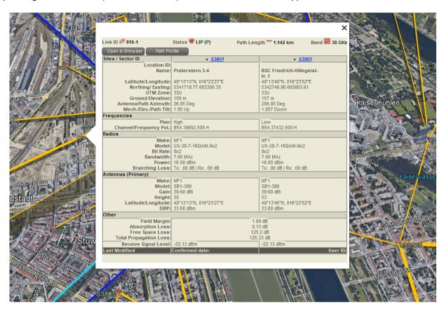
Click on Path Profile button to see profile of selected link. Profile data are obtained online, 100% of 1<sup>st</sup> Fresnel-zone and Line-of-Sight between sites are displayed. Actual height data on profile and marker on overlay map will be show when cursor moves along profile.
