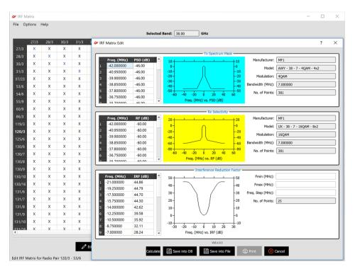
NOTE: If you use the C/I Method for evaluating interference objectives, you may use the Radio Import Utility to convert the IRF curves to C/I curves:
