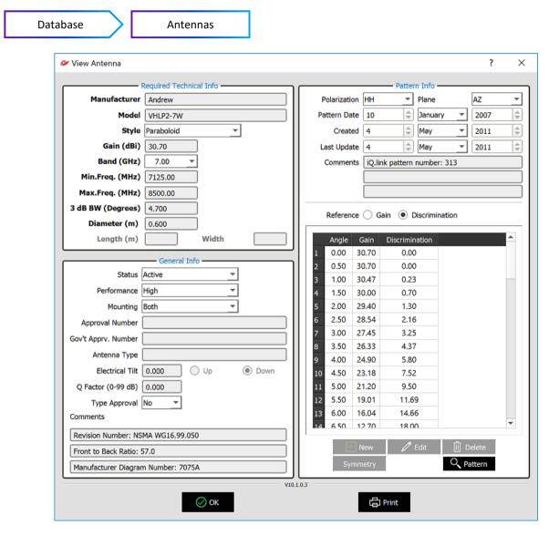
In Pattern Info tab HH, HV, VH, VV patterns can be selected by clicking Polarization drop down box.
