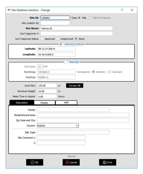
NOTE: Mandatory fields for a site are the ID, Name and a set of coordinates (labeled in bold). If you leave ground elevation empty, or set it to 0, the ground elevation will be automatically determined from the GIS data at the given location.
