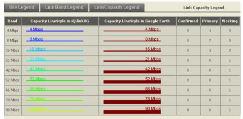
NOTE: The bitrate database is used to classify microwave link bitrates based on the capacity of the radio used and the number of channels assigned to each microwave link. The information stored through this interface is used by Network View to determine the total bitrate of each microwave link.
