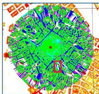
3.5 GHz RSL Plot using traditional ITU loss model
